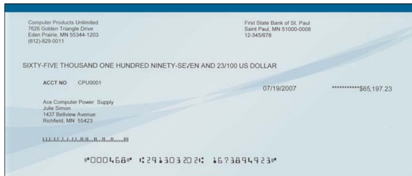
The MICR line on a check allows the check information to be automatically read for quicker processing.
